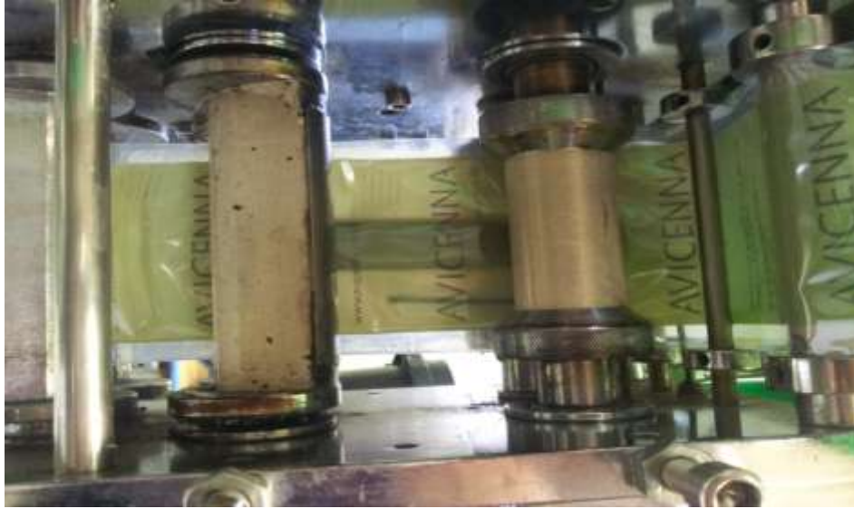
The empty plastics being run through the packing machine
