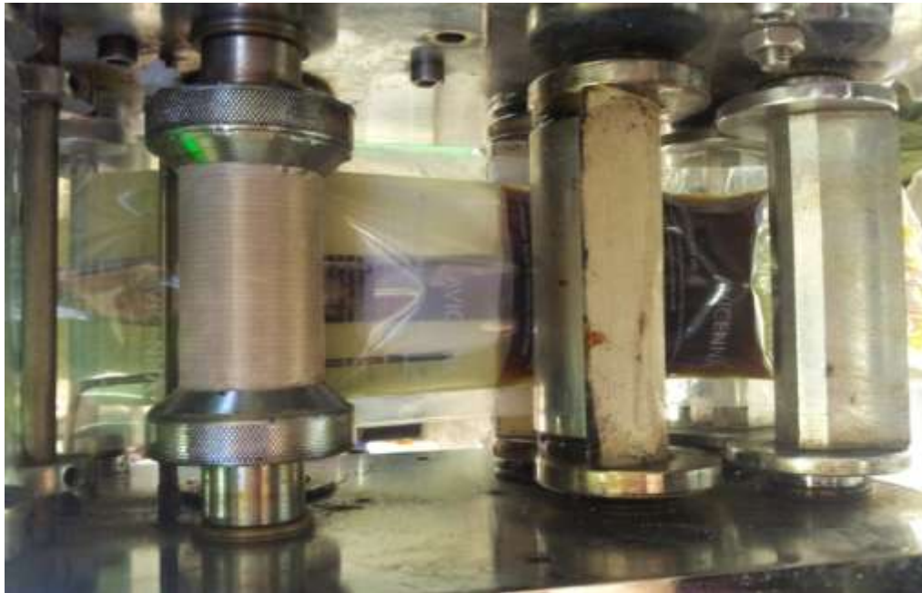
The hot herbs being piped into the empty plastics in the packing machine
